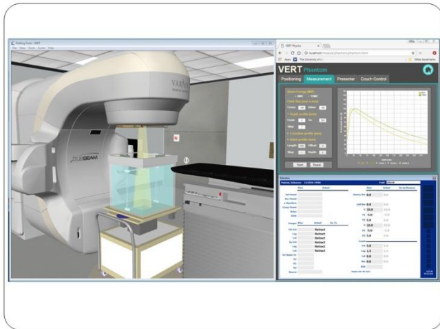
Fig. 2 Image of the full-size, 3D room screen set-up for the interactive demonstration and plotting tank measurements. Tutor and students would use mouse and machine specific hand pendant controls for set-up and measurements
