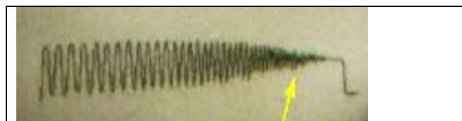
Fig.5 Contrast inversion manifested at the denso-profile of test object with gradually increasing spatial frequencies (plot of pixel values along a line through the image of the test object). The arrow indicates the Contrast Inversion.
