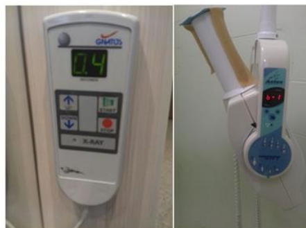
Figure 1: On the left, a Gnatux machine with selectable times. On the right, an Astex machine with a preset menu
