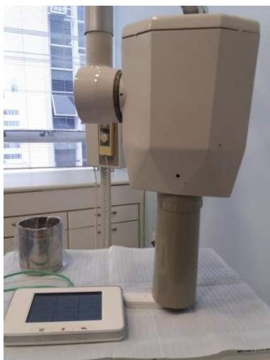
Fig. 2 Experimental arrangement adopted. Solid-state detector positioned at the exit of the X-ray tube.
