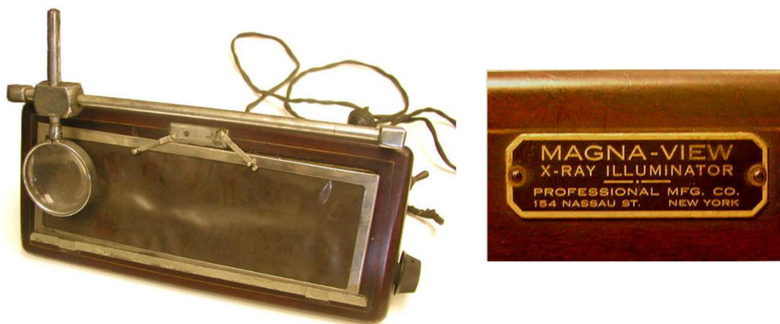
Fig. 69 X-ray film illuminator; estimated manufacturing date 1950s. The level of illumination by the incandescent bulb was adjustable. Figure and information provided by the Oak Ridge Associated Universities (ORAU) Health Physics Historical Instrumentation Museum Collection under a non-transferable, non-exclusive, limited license [156].
