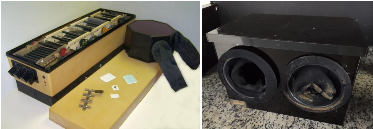
Fig. 37 Left: Litton automatic dental film processor with daylight loading. Courtesy of D. Bednarek (University at Buffalo). Right: Manual development using a lightproof glovebox.
