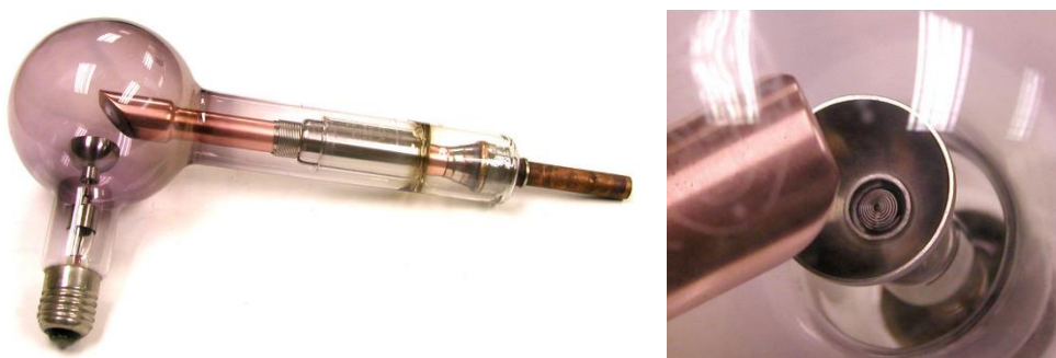
Fig. 19 Coolidge-type RD (Radiator Dental) dental x-ray tube (Victor X-Ray Corporation), manufactured ca. 1926-1932. The right-angled design was suited for dental radiography, allowing close tube positioning. The cathode, which was closest to the patient, was grounded, and the high-potential anode was deliberately positioned away from the patient, according to the original 1919 patent [54]. Left: the spherical part of the tube shows the focusing cup and the target (embedded in a slanted copper block). Right: close-up of the focusing cup, showing the tungsten filament. When in use, a finned metal radiation was placed over the copper rod for heat dissipation (not shown on figure). This type of tube was self-rectifying, meaning that it could be directly attached to an induction coil or transformer. Figure and information provided by the Oak Ridge Associated Universities (ORAU) Health Physics Historical Instrumentation Museum Collection under a non-transferable, non-exclusive, limited license [55].
