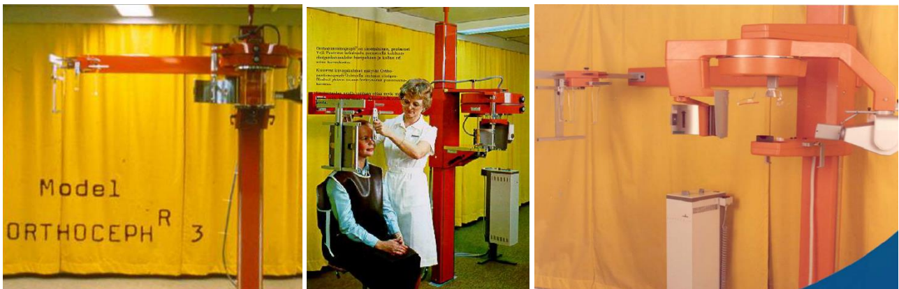
Fig. 46 Left and middle: the Orthopantomograph OP3 (1972-1978, Instrumentarium, Tuusula, Finland) combined panoramic and cephalometric radiography. Over 10 000 units were produced. Right: the Orthopantomograph OP5 (1978-1983, Instrumentarium) featured new patient positioning tools and an improved imaging geometry. Over 20 000 units were produced. Courtesy of Instrumentarium Oy and J. Mudrak.
