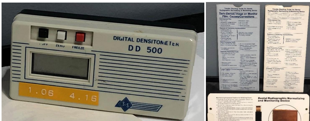
Fig. 39 Left: Digital densitometer (DD500 S&S X-Ray Products). Right: troubleshooting guide for dark and light radiographs. Courtesy of S. Anamali (University of Iowa).
