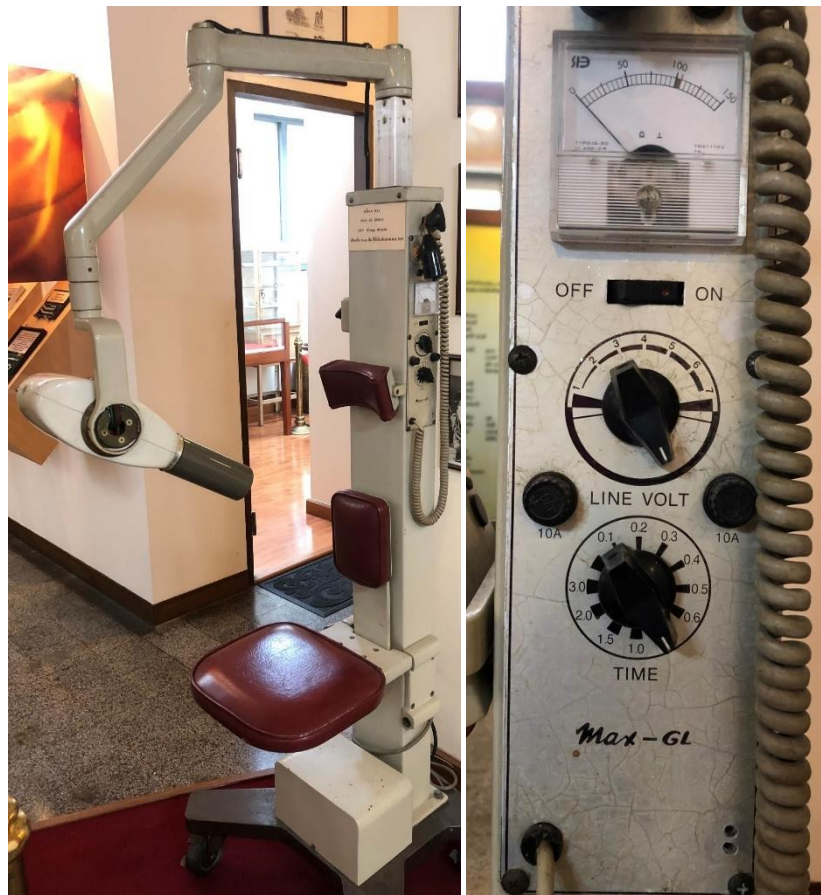
Fig. 26 MAX-GL dental X-ray unit (South Korea, ca. 1972) with built-in chair. Courtesy of P. Pittayapat (Chulalongkorn University).
