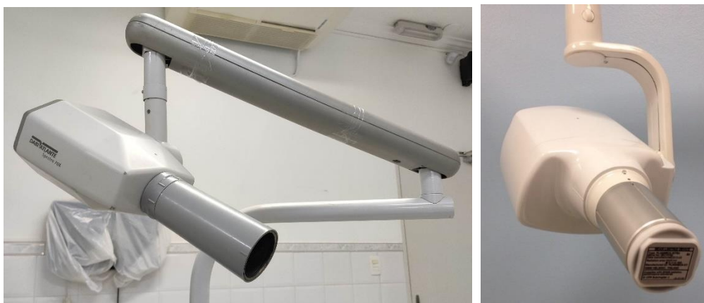
Fig. 29 Intra-oral X-ray tube with circular (left, ca. 2005) and rectangular (right) collimation. The use of circular collimation is still prevalent, despite the considerable dose reduction obtained using rectangular collimation [61-64]. Right figure courtesy of K. Horner (University of Manchester)
