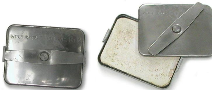
Fig. 32 Wolf X-ray intra-oral cassette for occlusal radiography (ca. 6.4 x 8.3 cm). The cassette appeared in a 1955 catalog, which mentioned an exposure time of 1.5-2 s. Figure and information provided by the Oak Ridge Associated Universities (ORAU) Health Physics Historical Instrumentation Museum Collection under a non-transferable, non-exclusive, limited license [74].
