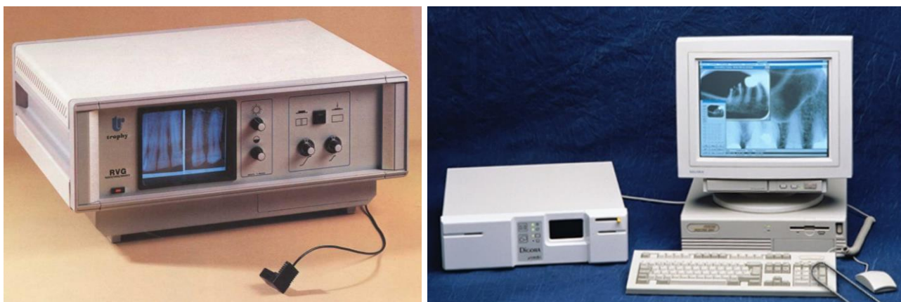
Fig. 40 Left: the RadioVisioGraphy a digital charge-coupled device (CCD) intra-oral detector (1987, Trophy Radiologic, France). Courtesy of A. Wenzel, Aarhus University. Right: The DIGORA ('DIGitalORAI') system intraoral imaging system using storage phosphor plates (1994, Soredex, Tuusula, Finland). Courtesy of Soredex Oy and J. Mudrak.
