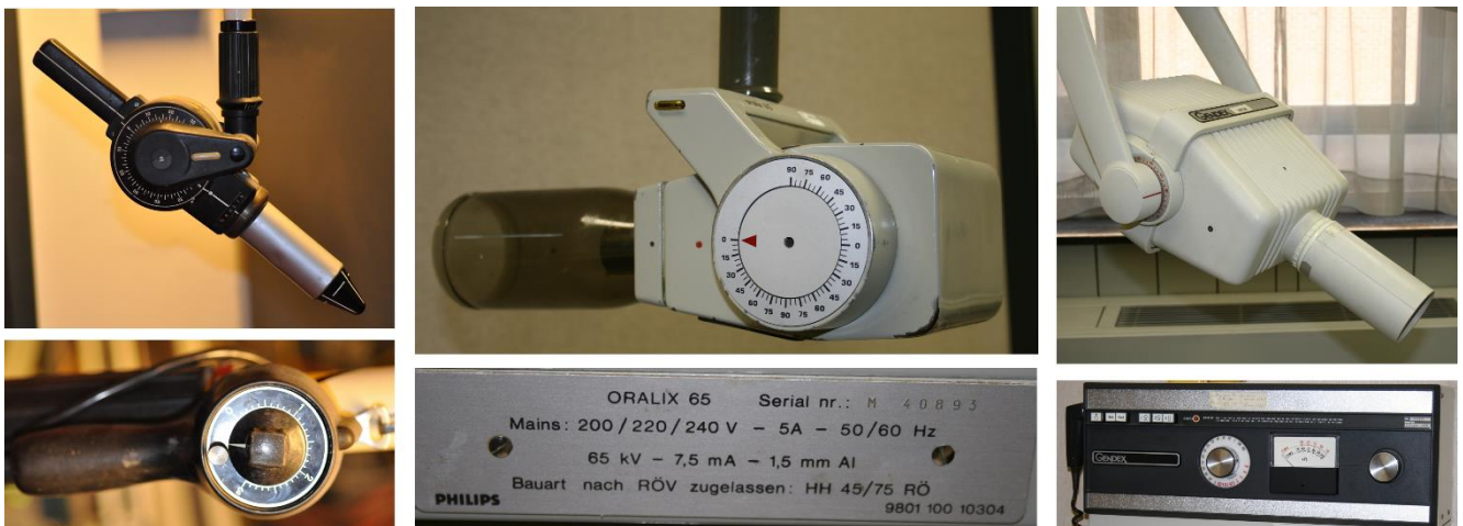
Fig. 27 Oralix 50 (left; ca. 1960s-1970s) and Oralix 65 (right; ca. 1984) intra-oral X-ray units (Philips, The Netherlands). The model number seemingly referred to the kV at stability ( i.e. not the kVp) of the tube [61]; a '45' model was also produced. Absorbed dose to the skin inside the primary beam ranged between 3.3 mGy and 9.7 mGy for these two units [61]. Right: Genex GX 1000 (ca. late 1980s). Courtesy of J.K.M. Aps (University of Western Australia).
