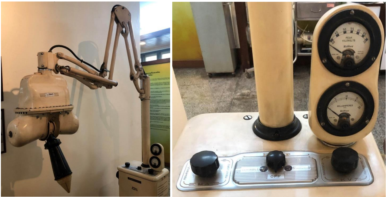
Fig. 24 Ritter Dual-X unit (ca. 1950). Notice the double-cone design of the tube head, combining a longer source-skin distance with a position indicating device. Courtesy of P. Pittayapat (Chulalongkorn University).
