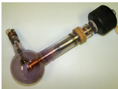
Fig. 17 Coolidge-tube (10 mA), ca. 1922. Courtesy of D. Bednarek (University at Buffalo).
